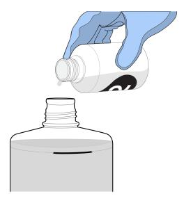
**Note:** Keep the Ion  $PGM^{TM}$  Hi- $Q^{TM}$  Sequencing W2 Solution bottle to scan the barcode during the initialization procedure.
