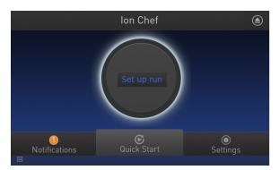
**3.** Touch **Step by Step** to have the instrument lead you through the instrument setup, or touch **Quick Start** to skip the instrument setup screens.
