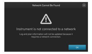
See Appendix C, "Ion Chef<sup>™</sup> and Torrent Server network setup" to troubleshoot your network connection. Touch the close symbol X in the upper right corner to return to the Data Destination screen. To bypass a Torrent Server or network connection and proceed with the run, touch OK, then select the template size for your run on the next screen:
