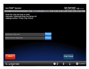
**4.** When prompted by the instrument, ground yourself by touching the grounding plate next to the chip clamp on the instrument, replace the cleaning chip in the chip socket with the chip to be sequenced, close the chip clamp, then touch **Next**.
